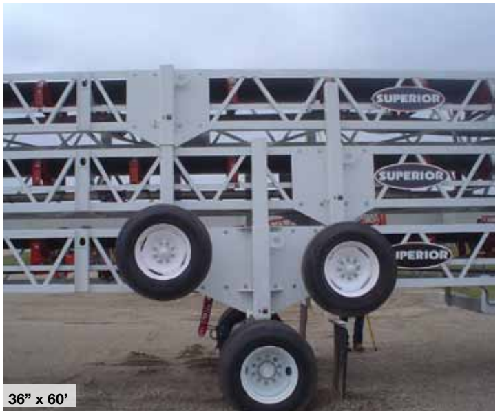
Piggyback conveyors' adjustable height legs can adjust to uneven terrain independently
